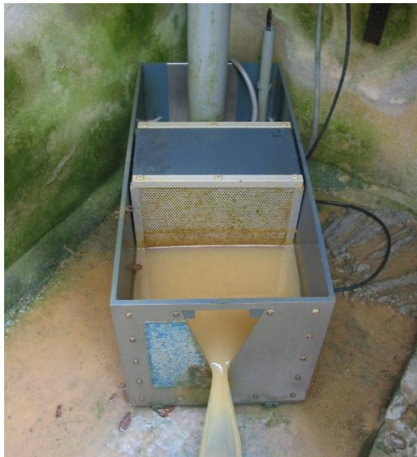
Figure 8: Water collector. Drainage and runoff collectors for measuring the flow rates and collecting water samples (Selected papers from ARVALIS No.11).
