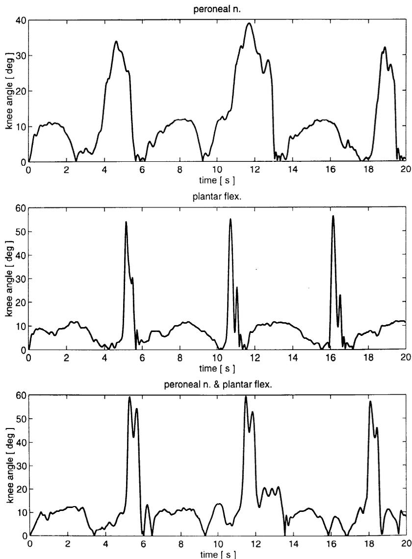
**FIG. 3.** The knee goniograms shown were made during walking with peroneal nerve stimulation (**upper trace**), with stimulation delivered to the ankle plantar flexors (**middle trace**), and with stimulation of the ankle plantar flexors and peroneal nerve (**bottom trace**).
