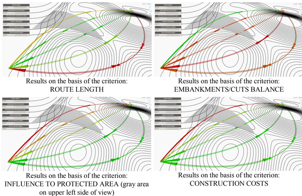
Figure 6: Results of the optimization of the test model for different optimization criteria (criteria 1 - 4)
