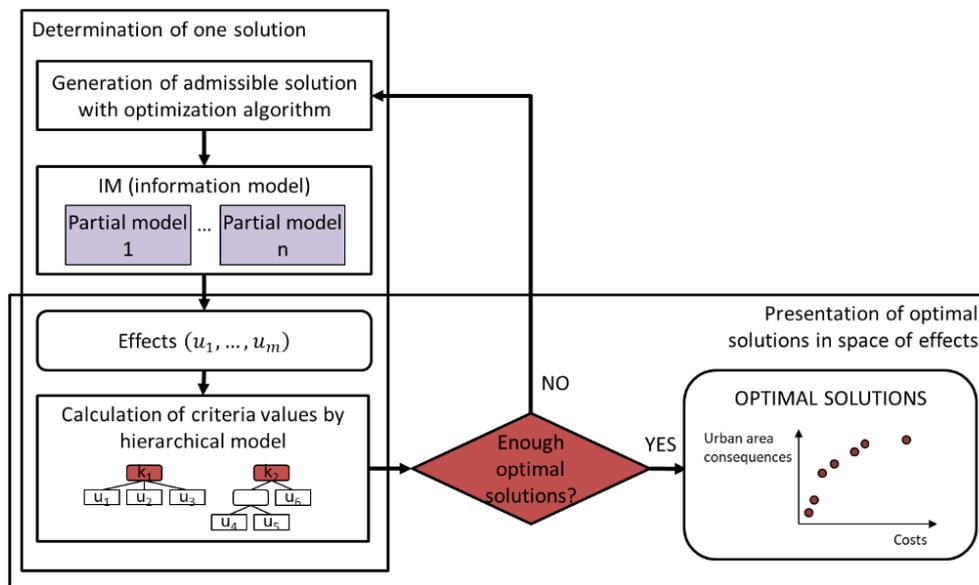
Figure 7: Multi-objective optimization in the proposed process
