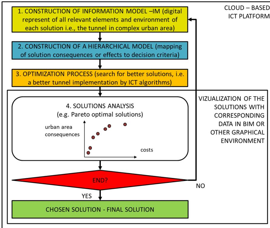
Figure 2: Steps of the proposed infrastructure design process
