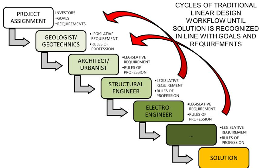
Figure 1: Traditional design process workflow
